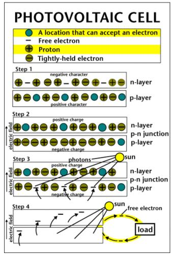
The P-N junction makes solar energy possible by creating an environment in which the maximum amount of electrons are freed by the sun's energy and forced to travel through an electric field to create usable electricity. <sup>15</sup>
